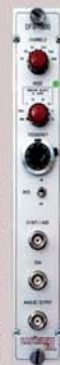
DFG-1000 Standard Model Sine, Constant Acceleration (triangle), Constant Velocity (with different slopes), control signals 128 - 4096 channels 1 - 100 Hz
